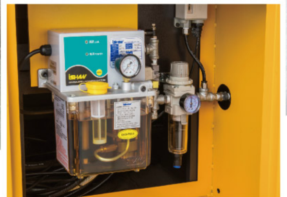
Automatic lubrication unit.
