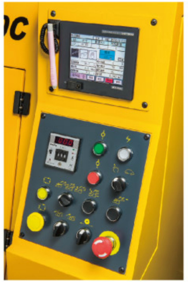
Friendly And Easy To Operate Touch Screen • Expandable built-in cutting data library. • Key NC parameters can be turned/set in Service-Maintenance pages. • Self-diagnose capability. • Fully digitized data input structure.
